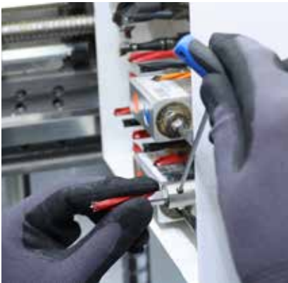
Weldon change system For a drill bit change with tools.
