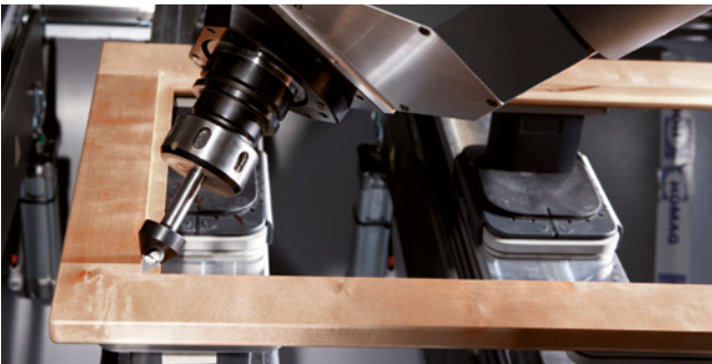
Square corner routing for a glass rebate
