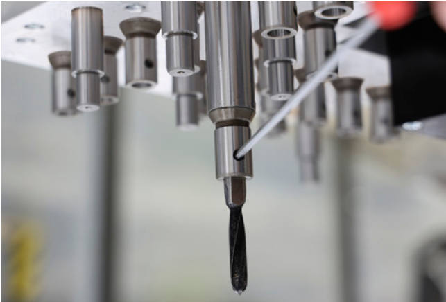
Weldon change system for a drill change with tools
