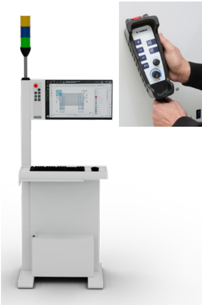
Operator terminal ▪ powerControl with powerTouch ▪ 24" Full-HD multitouch display ▪ USB frontside bus ▪ Ethernet connection 10/100 Mbit ▪ Inklusive flexible mobile handheld terminal for easy operation
