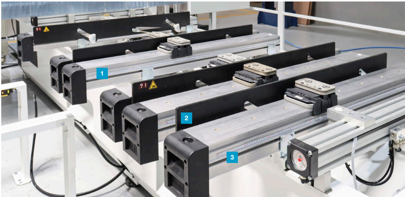
3-4 Axis machine console system suitable for 50 mm height Vacuum cups
