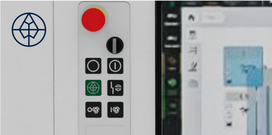
ecoPlus – energy saving function ▪ Simple activation of the stand-by mode ▪ Vacuum pump is switched off (savings of up to 12%) ▪ Reduction of compressed air (savings of up to 6%)
