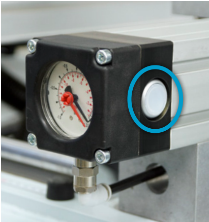
Button for program start Each one at the left and right hand stop profile act as program start for the processing.
